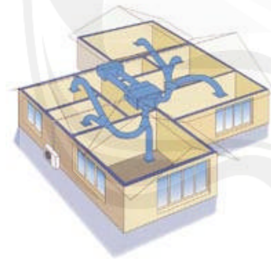
Gambar 6.24 System Ducting Sumber : http://www.heatpumpsinfo.co.nz
