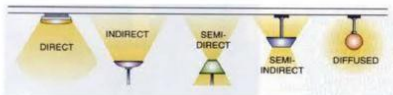
Gambar 2.9 Lima Teknik Distribusi Cahaya Sumber : Philips Methods of Light Dispersement
