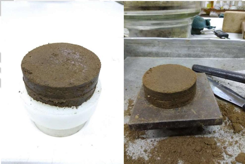
Specimens After Direct Shear Test
