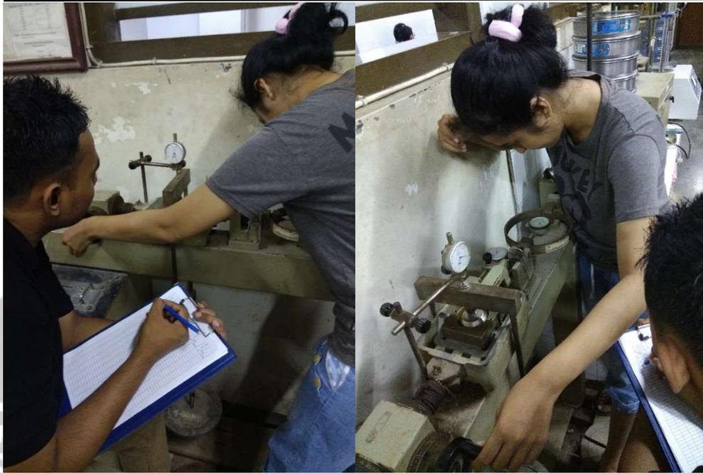
Conducting Direct Shear Test and Taking Test Data
