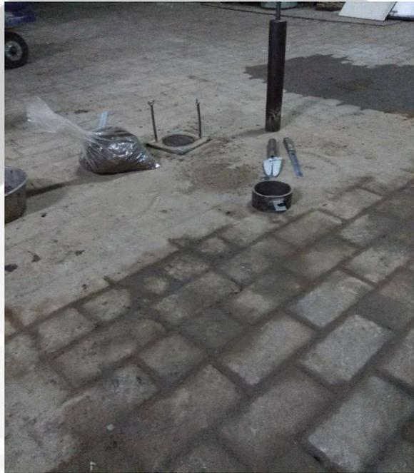
Standard Proctor Test Preparation
