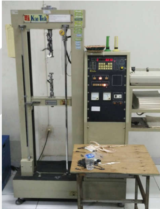
Gambar 3.12. Universal Testing Machine
