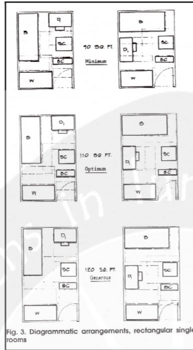
Fig. 3. Diagrammatic arrangements, rectangular single rooms
