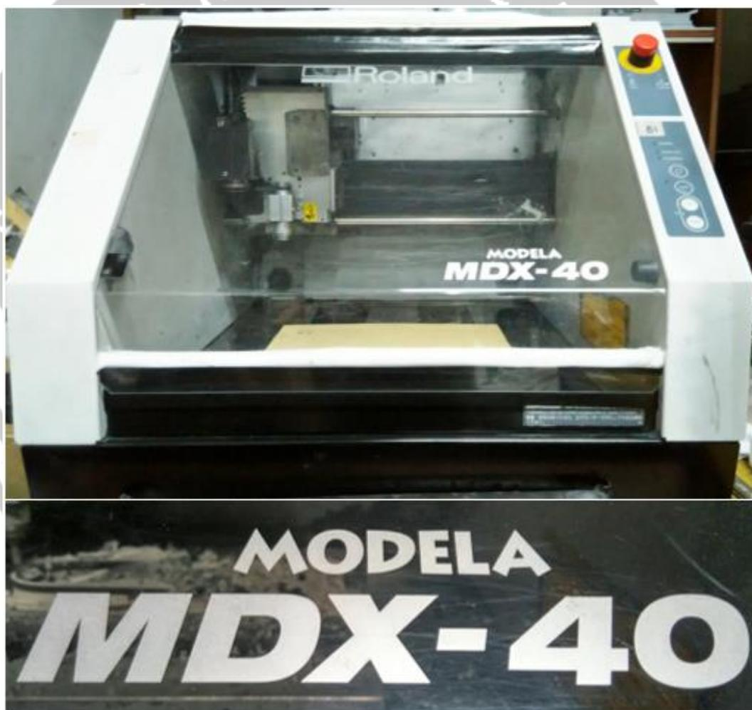
**Gambar 2.11. Mesin *CNC Roland Modela MDX – 40R***
