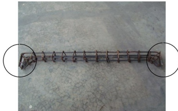
Fig. 3 Detail of reinforcement column specimen
