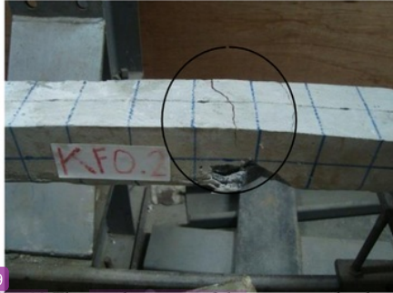
Fig. 10 The crack pattern of the unwrapped column
