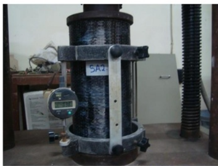
Fig. 4 Modulus elasticity testing of cylinder concrete
