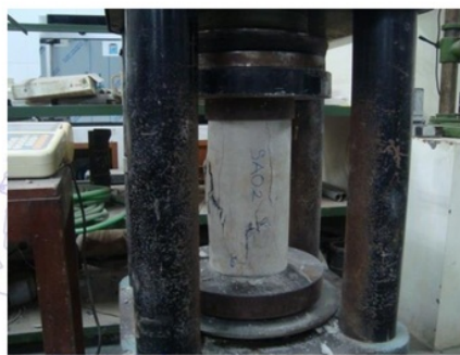
Fig. 5 Compressive strength testing of cylinder concrete
