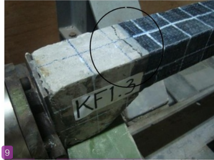
Fig. 11 The crack pattern of the wrapped column
