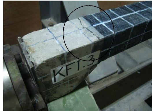
Fig. 11 The crack pattern of the wrapped column
