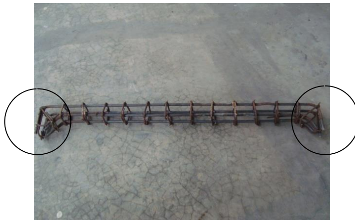
Fig. 3 Detail of reinforcement column specimen
