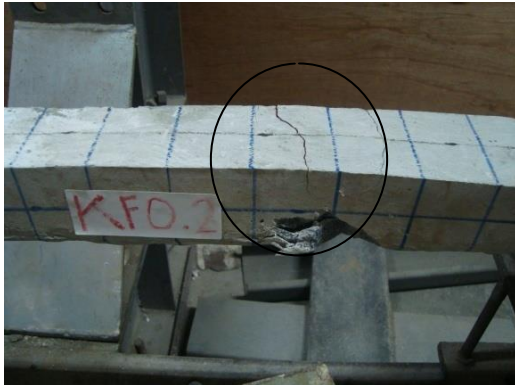
Fig. 10 The crack pattern of the unwrapped column
