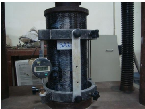
Fig. 4 Modulus elasticity testing of cylinder concrete
