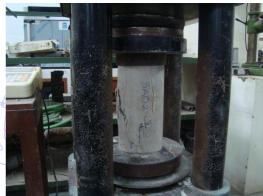
Fig. 5 Compressive strength testing of cylinder concrete
