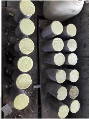
Proses Caping Beton
