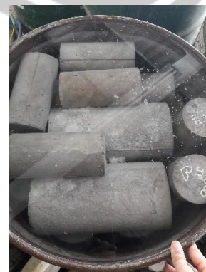
Proses Curing Beton
