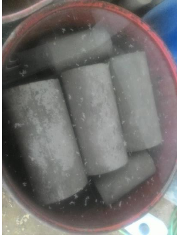
Proses Curing Beton
