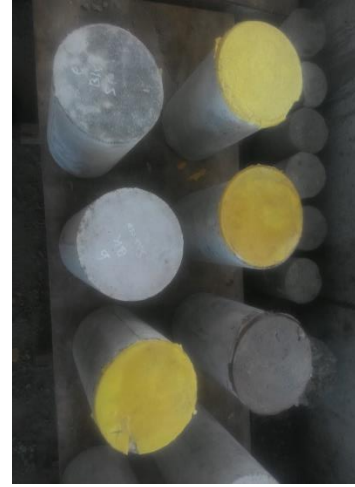
Proses Capping Beton
