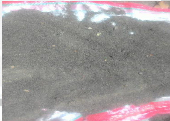
Proses SSD Agregat Halus
