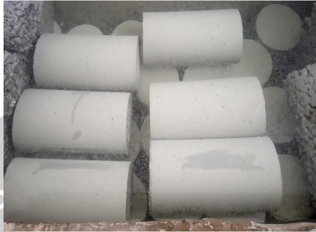
Proses Curing Beton
