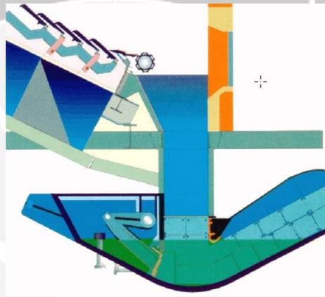
**Gambar 2.21** Detail slag discharge
