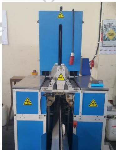
Figure 3.27 Casing In Machine
