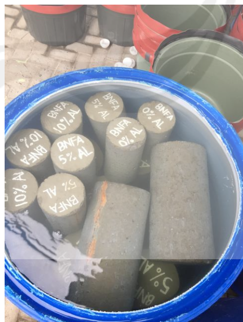
Gambar 4. Proses Curing Air Laut
