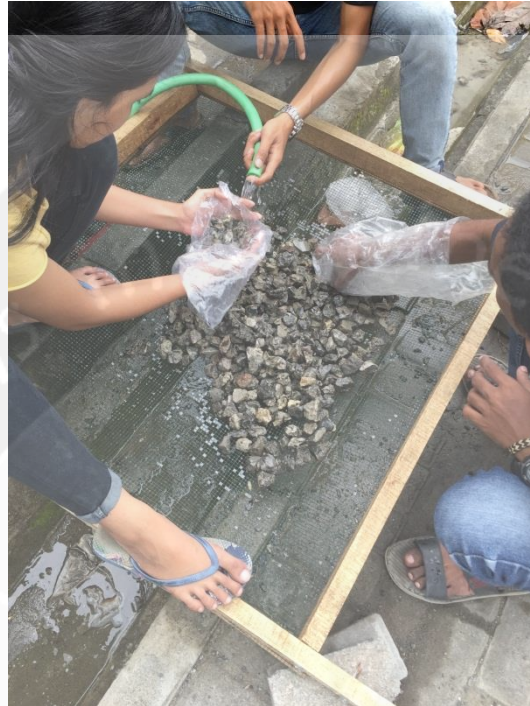
Proses Pencucian Agregat Daur Ulang
