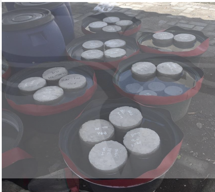
Proses Curing Beton Silinder
