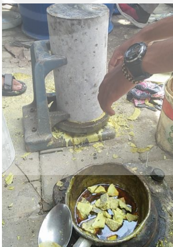
Proses Capping Beton
