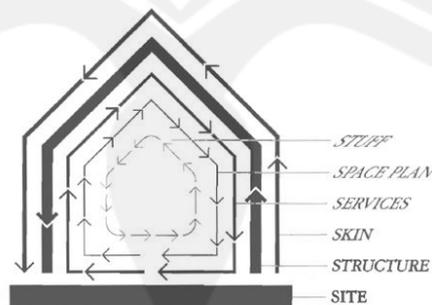
Gambar 3.1 *Building Layer Diagram*
