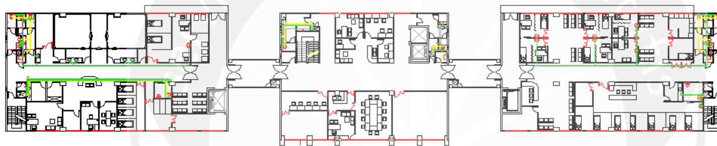
Gambar distribusi air buangan lantai 3
