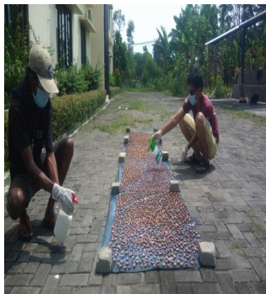
Proses Waterproofing Treatment Keramik
