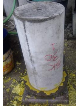
Proses Capping Silinder Beton
