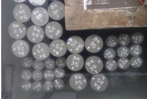
Proses Curing Silinder Beton
