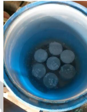
Proses Curing Beton
