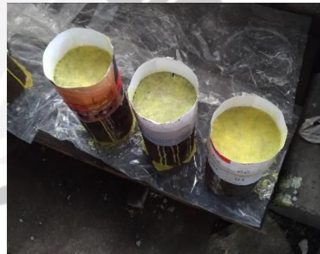
Proses caping beton
