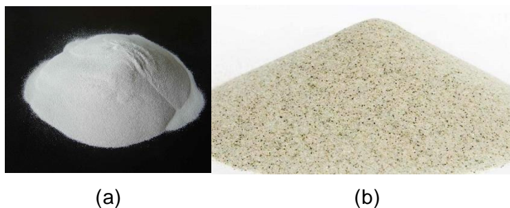
Gambar 2.2. Bahan dasar porselen. (a)alumina, (b)silica.
