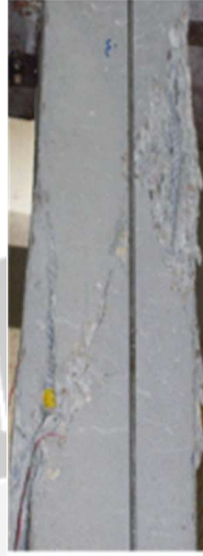
Figure 2.2. Specimen C4 failure in experiment.
