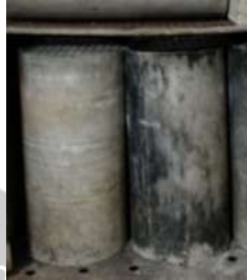
Proses Dry Curing Beton Geopolimer
