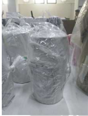
Proses Ambient Curing Beton
