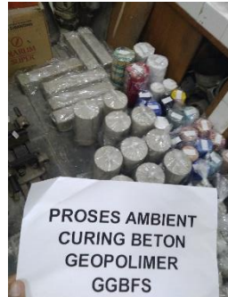
Proses Ambient Curing Beton
