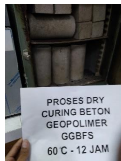
Proses Dry Curing Beton Geopolimer
