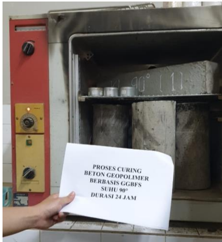
Curing Oven Suhu 90°C
