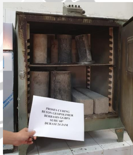
Curing Oven Suhu 60°C
