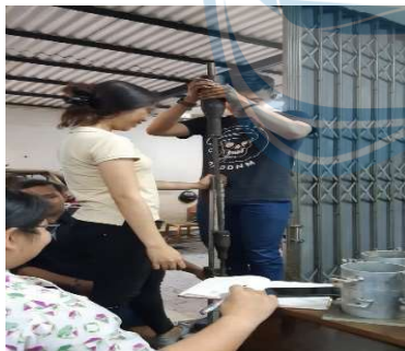
Figure A.13 DCP Test
