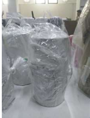
Proses Ambient Curing Beton
