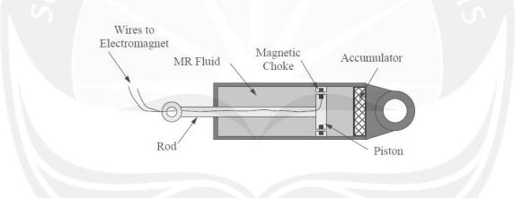
Fig.2.1 Schematic of MR damper
