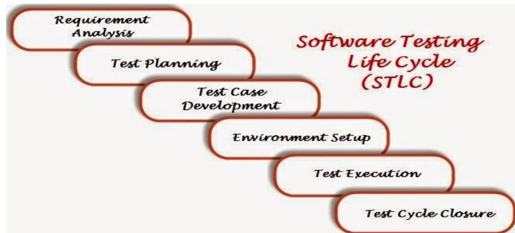
Gambar 3.2 Software Testing Life Cycle(STLC)
