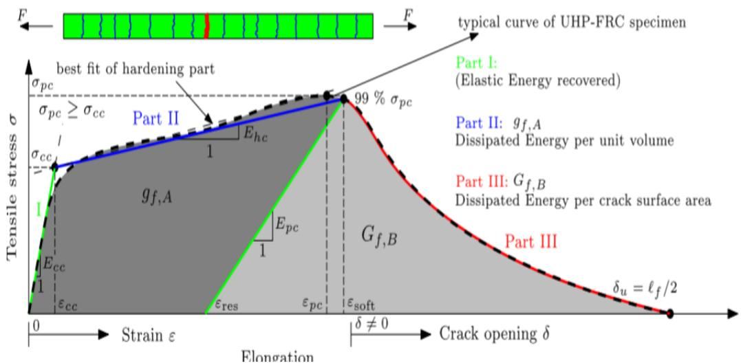
**Figure 2.2** UHPFRC Stress-Strain Graph Under Tension (Wille et al, 2014)
