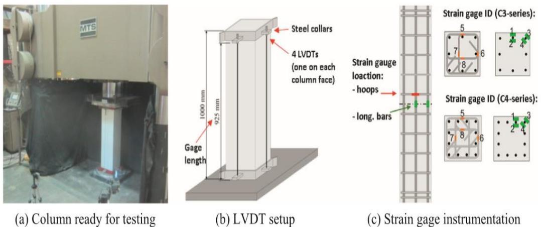
**Figure 2.4** Column Instrumental and Test Setup for Compression
