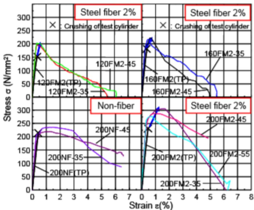
**Figure 2.3** Result of Column Compressive Test (Sugano et al., 2007)
