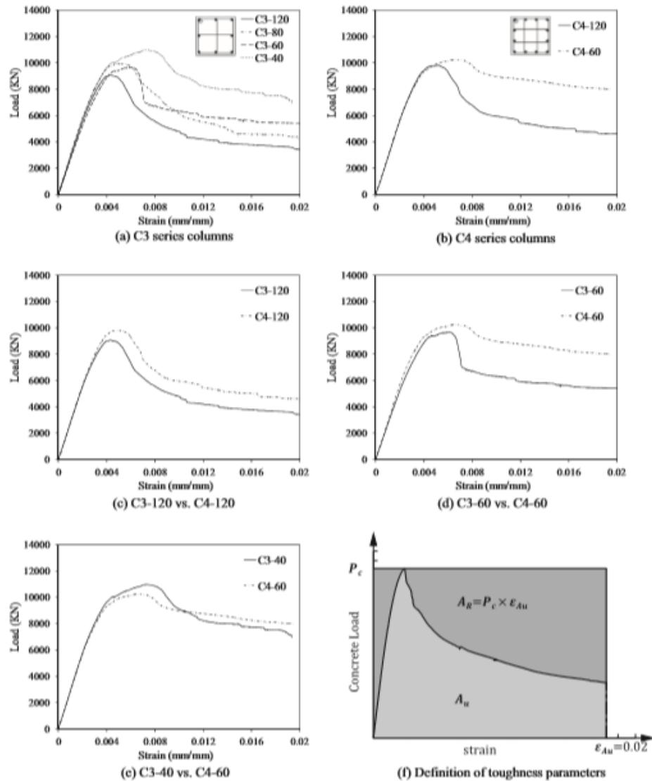
**Figure 2.5** Load-Strain Result of UHPFRC Columns (Hosinieh et al., 2015)
