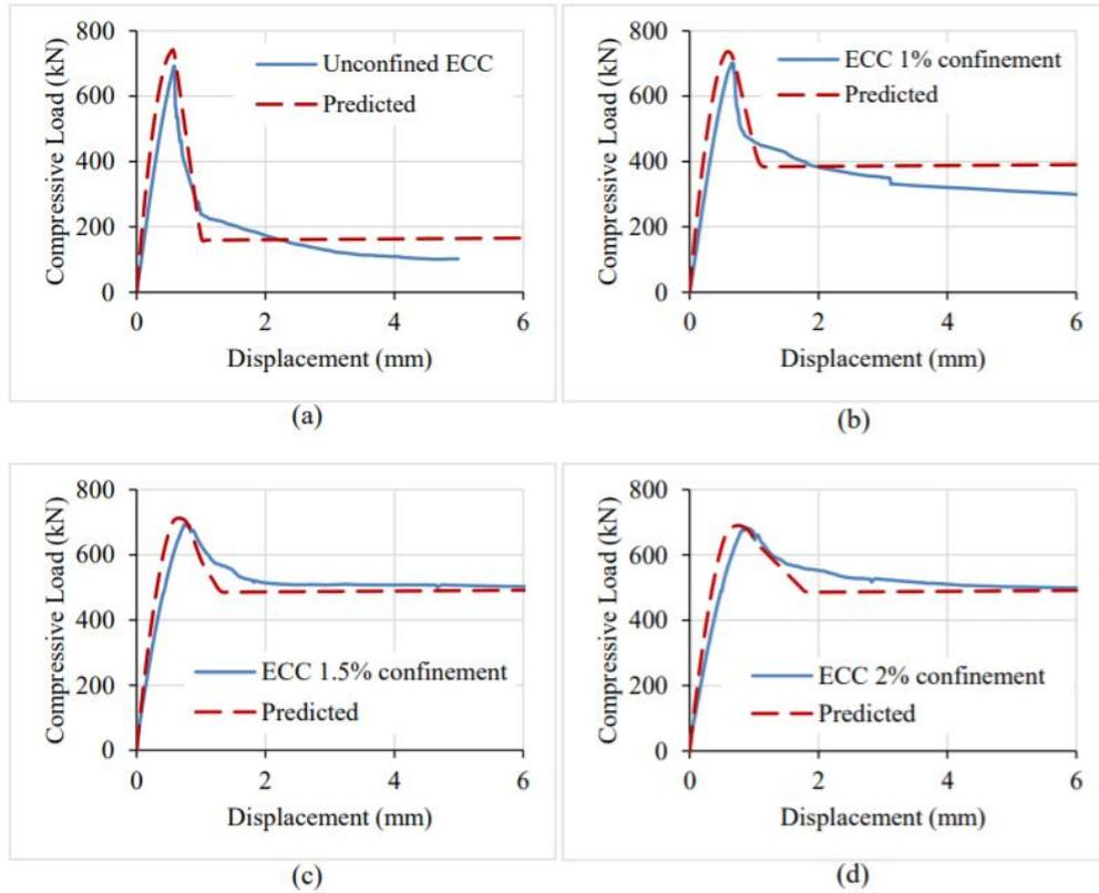
**Figure 2.6** Load-Displacement Result of ECC columns (Wong, 2018)
