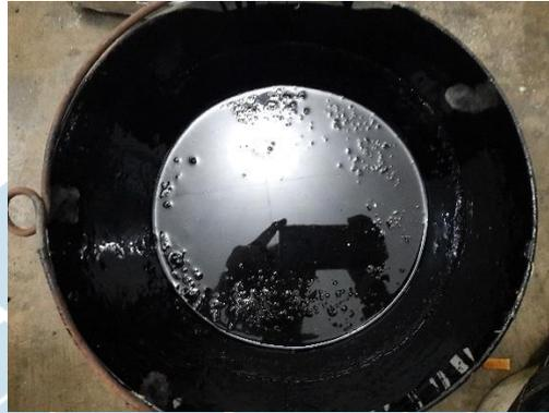
Gambar 3.2 Aspal penetrasi 60/70
