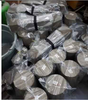
Proses Ambient Curing Beton
