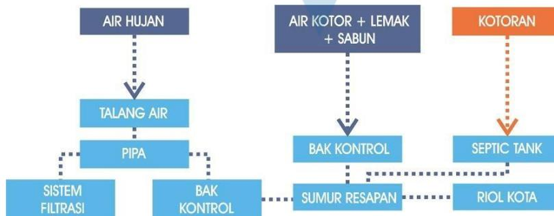
**Gambar 6.9** Diagram Analisis Sistem Distribusi Air Kotor
