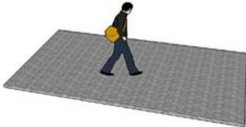
Figure 3.2 Level of service of sidewalk standard A
