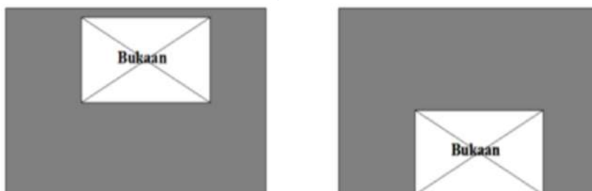
Figure 2.4 Illustration of checking type 3 horizontal irregularity (SNI 1726:2019)
