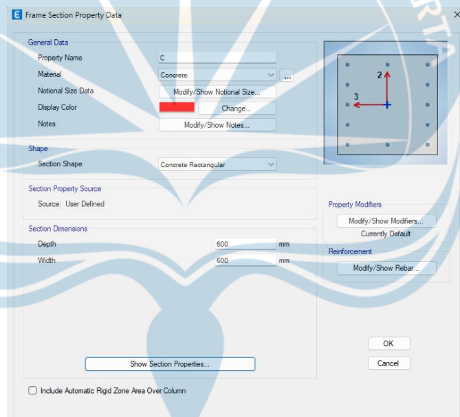
Figure 2.10. Frame Section Property Data of Column
