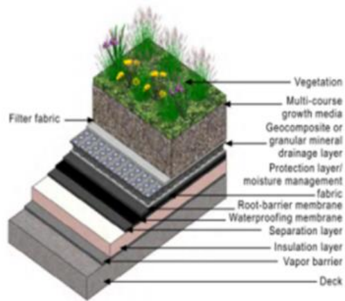
Gambar 3.9.2.2 Tipe Green Roofs Semi Intensive
