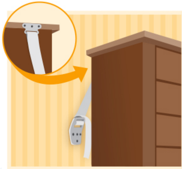
Gambar 2. 8 Mengamankan Perabot dengan Pengikat Sumber: (6 Tips for Installing Furniture Restraints to Prevent Tip-overs, n.d.)
