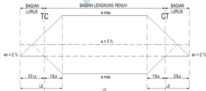
Gambar 2. 4 Diagram Superelevasi Full Circle ( Sumber : Hendarsin,2000)
