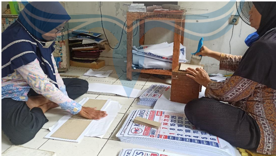
Gambar 1.4. Proses Finishing (Pengeleman Hard Cover)
