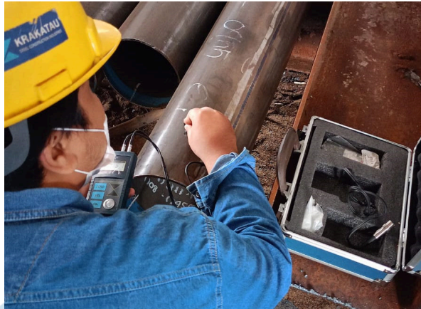
Figure 2.7 Material Thickness Checklist of PLN JTM 9/200 Electric Pole
