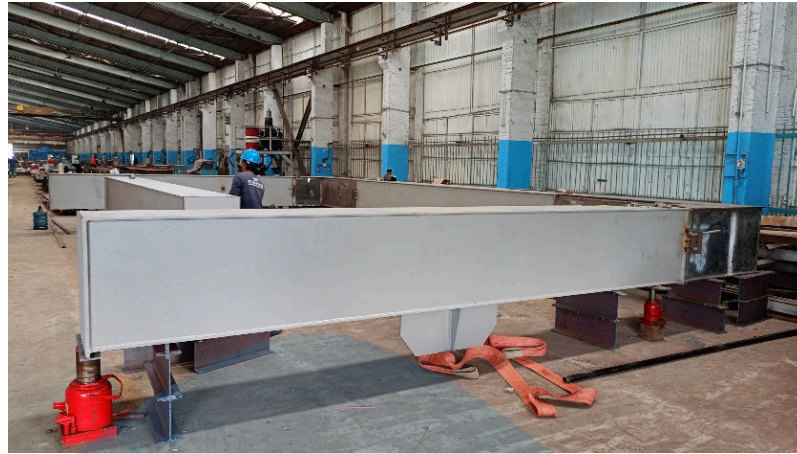
Figure 2.16 Coal Hopper Plate Girder Checklist
