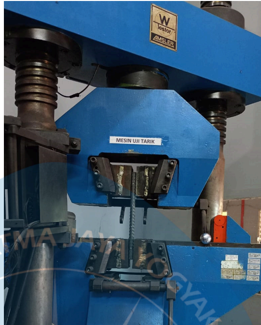
Figure 2.22 Steel Bar Tensile Test
