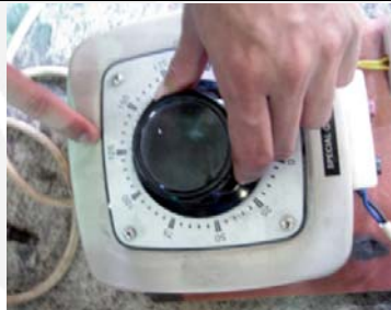
Figure 6.10 Set the regulator at 125 volt to get constant speed
