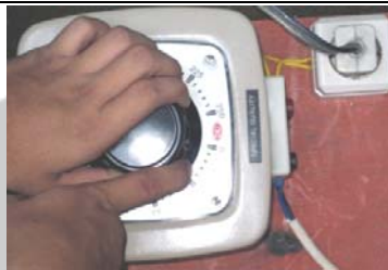
Figure 6.12 Set the regulator at 0 volt
