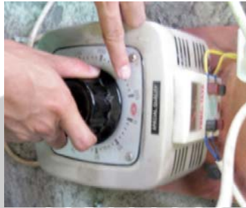
Figure 6.9 Set the regulator at maximum voltage to activate electric motor
