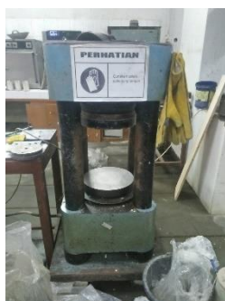
Compression Testing Machine
