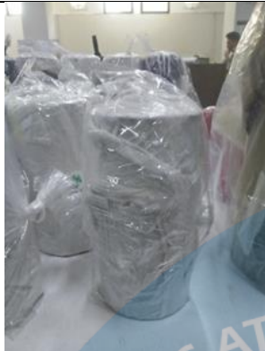
Proses Ambient Curing Beton
