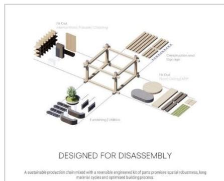
Gambar 2. 11 Disassembly design: BetaPort
