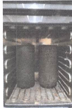
Proses Dry Curing Beton Geopolimer
