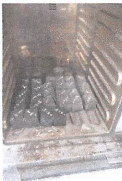
Proses Curing Mortar
