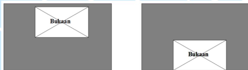
Figure 2.13 Horizontal Irregularity Type III
