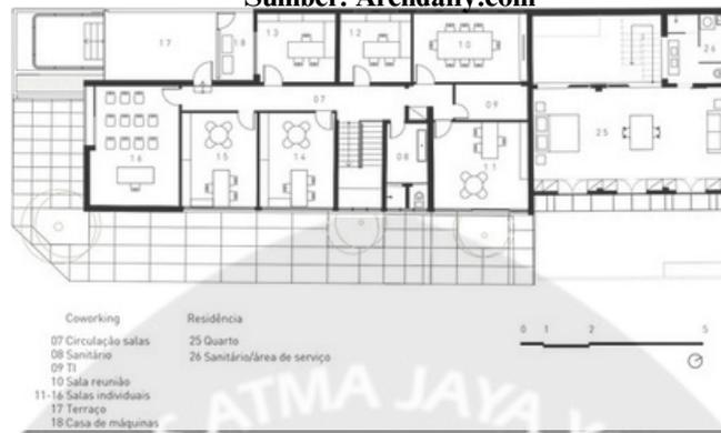
**Gambar 2.0 Denah Lantai 2 bangunan A Casa Coworking**
