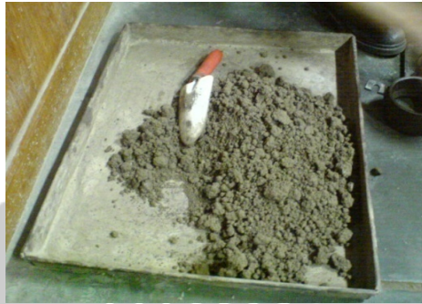
Figure 3.9 Clay + fly ash mixing
