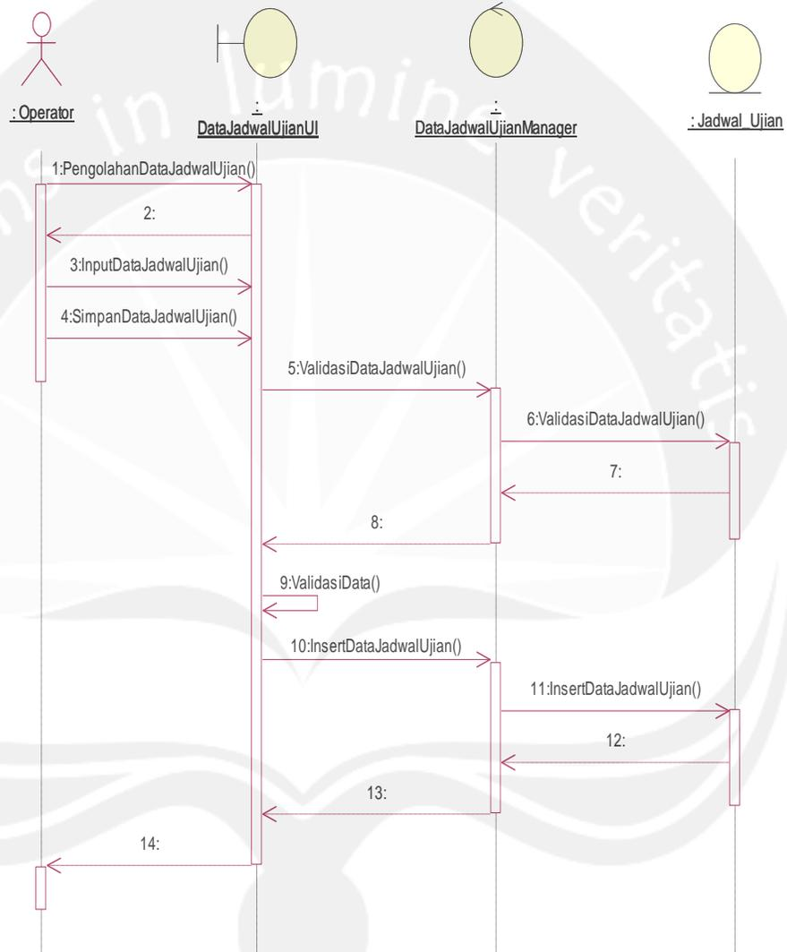
Gambar 23. Sequence Diagram Tambah Data Jadwal Ujian
